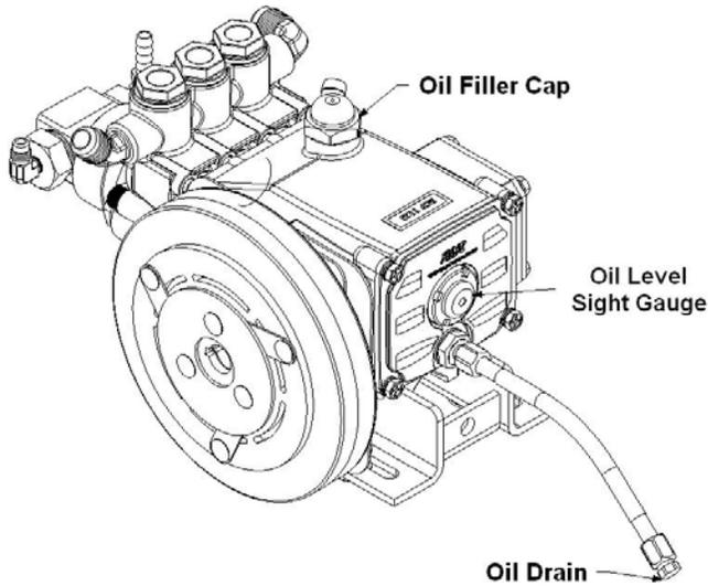
2. After the first **50 hours** of operation, change the crankcase oil with CAT Pump Crankcase Oil, (Part # 13-000). Change the crankcase oil every **500 hours** thereafter.
